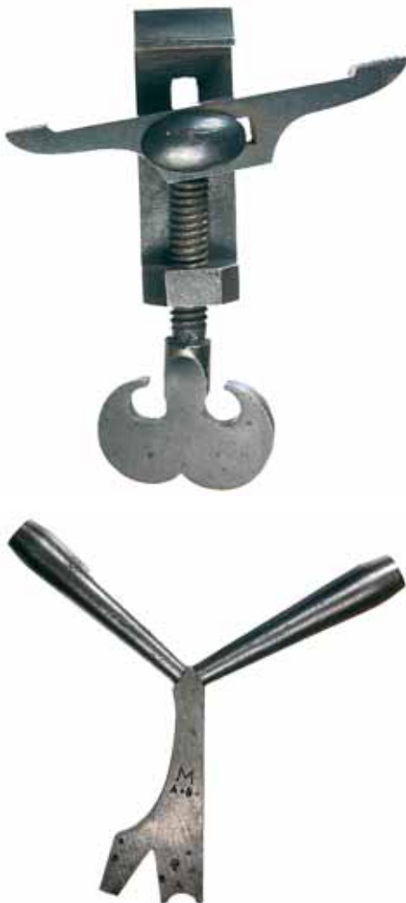
823* Combination percussion tool wrench , c1850s, for flintlock gun, marked on one side, 'M/A.S.'; also flintlock gun main spring vice. Very fine. (2) $100
