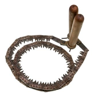
**WWII**, military chain-link, folding hand saw, with removable, fitted timber handles. *Fine*.
