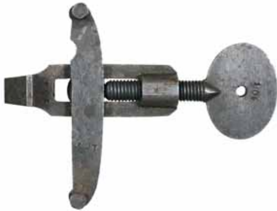
3013* Vintage gun mainspring vice , c1840, in steel for installing spring in a flintlock gun, impressed number 105 in two places and also impressed mark of Queen Victoria crown over W. Screw seized up, otherwise good very fine.
