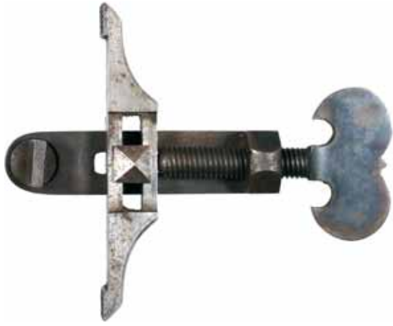
3012* Vintage gun mainspring vice , c1820, in steel for installing spring in a flintlock gun. Good very fine.
