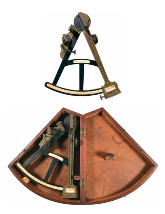
4112\* Sextant, brass fittings and ebony wood frame, ivory inserts with angles and measurements on the base of frame and arm, arm has a screw calliper brake, brass fittings hold colour filters, viewing lenses and mirrors as well as peep hole with sliding cover. *In good condition.*
